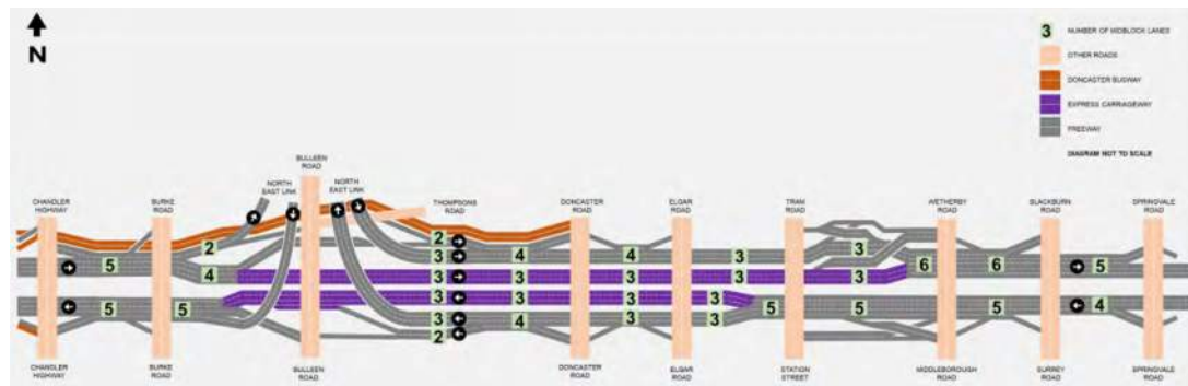
Figure 9-2: Proposed Through Lanes on Eastern Freeway East of Bulleen Road
