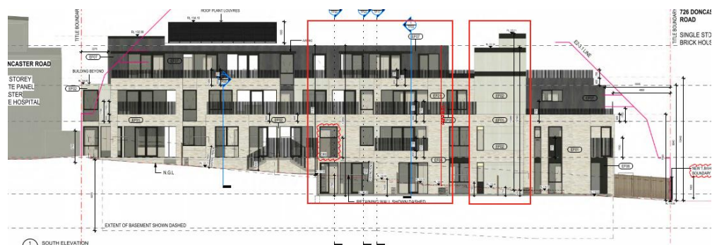
Figure 10: Four storey presentation to south (residential interface)
