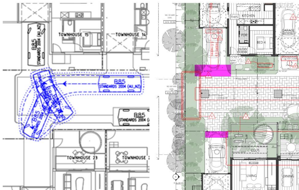
Figures: Extract from submitted swept path diagram; Annotated ground floor plan with recommended increases (pink) to common driveway
