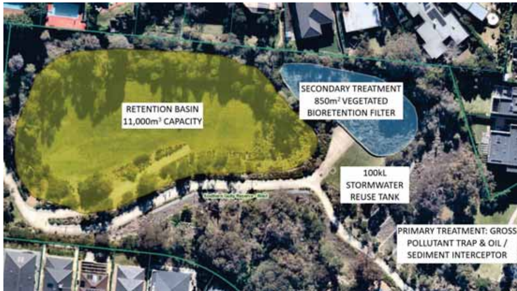
Figure 20: Tullamore Estate Retention Basin, Biofilta and Gross Pollutant Trap
