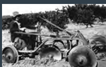
Stanley Crouch on his horse-drawn Petty Plough on the 'Dingley Dell' orchard, 1942. Designed locally by Frank and Herbert Petty using the T-Model Ford car chassis, it was made by Daniel Harvey Foundry in Box Hill
